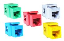
D-Link Category 6 keystone jacks are RJ45 8P 8C 50u jacks suitable for 22-26 AWG stranded and solid wire, compatible with both 110 & Krone punch down tools. They are available in universal labels Colour coded for T568A and T568B wiring schemes and fit in high density keystone patch panel. It supports IEC 60603-7-4 and complied with ANSI/TIA/ EIA-568-C.2 standard.
